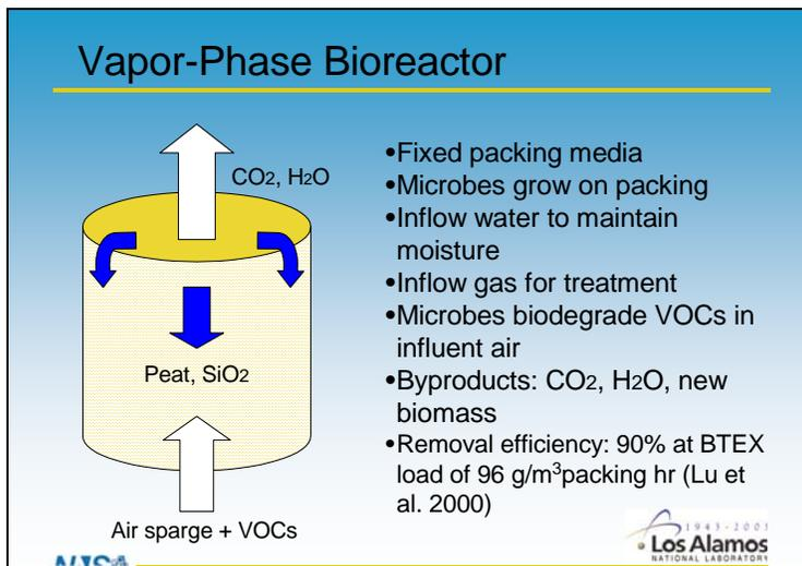
Air sparge vapor from the regenerating SMZ is routed through the Vapor Phase bioreactor. Microbes grow on support media and degrade volatile organic compounds. Removal efficiencies have been tested and found to be equal to or greater than published efficiencies of 90%.
