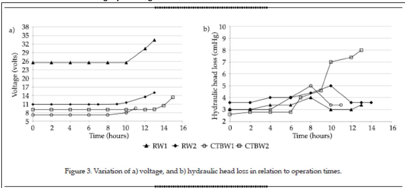
These upward trending curves clearly show the effects of passivation (above left) and sludge buildup (above right) in the Villegas-Mendoza reactor.
