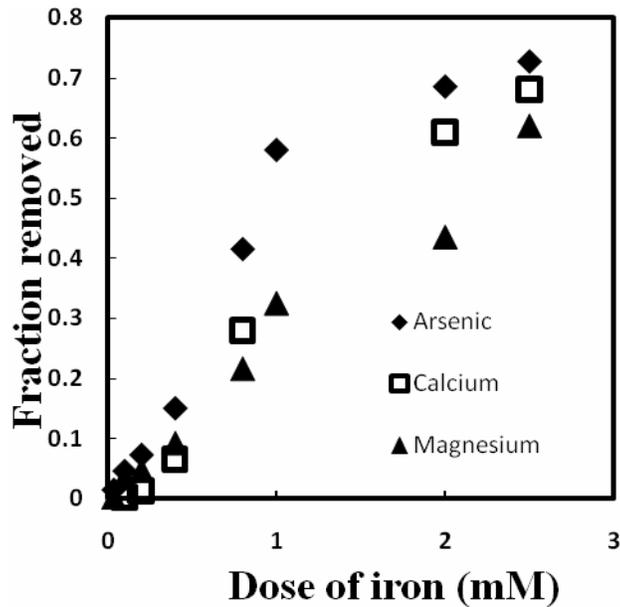
Figure 4- fraction of initial arsenic removed at 1.8 mM, calcium at 1.112 mM, and magnesium at 0.494 mM by iron blades as a function of coagulant dose at pH 7.
