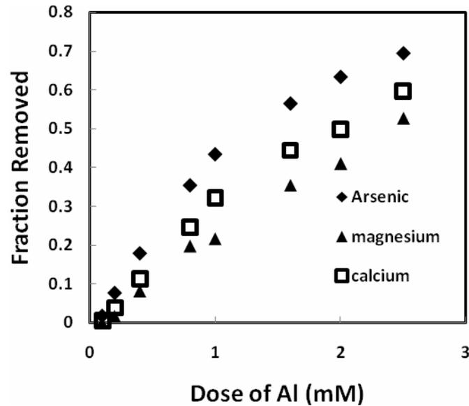
Figure 5- fraction of initial arsenic removed at 1.8 mM, calcium at 1.112 mM, and magnesium at 0.494 mM by aluminum blades as a function of coagulant dose at pH 7.
