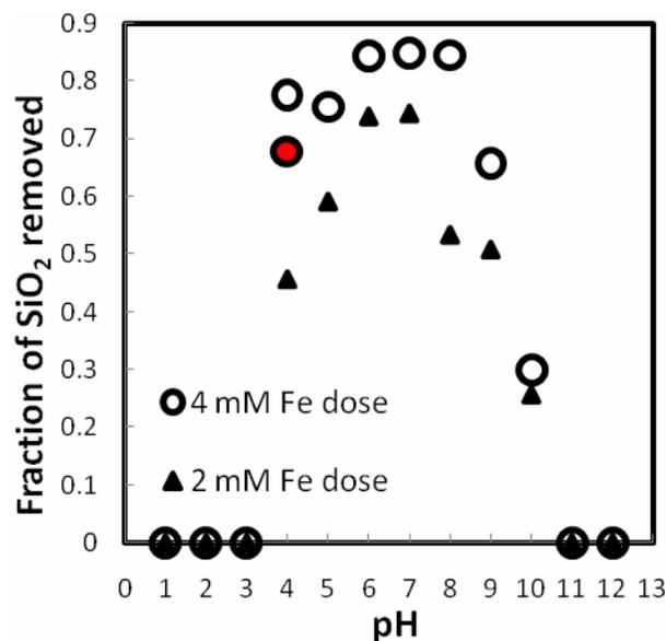
Figure 3- Fraction of SiO<sub>2</sub> removed vs. pH at 2 mM and 4 mM target Fe dose. The red mark is for the solution filtered with 0.47  $\mu\text{m}$  filter paper, while the rest of the solutions were filtered using 0.1  $\mu\text{m}$  filter paper. Initial concentration of silica is 1000 ppm.
