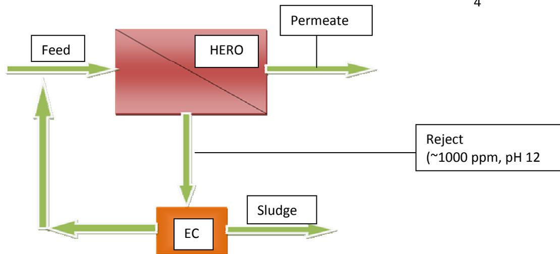
Figure 2- Illustration of the incorporation of EC technology in treating brine from HERO™
