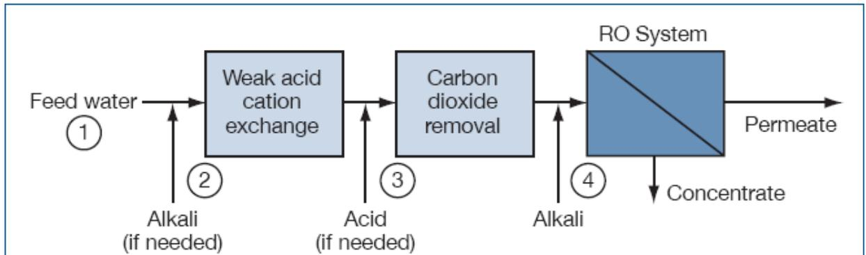
Figure 1 – Schematic of HERO™ system<sup>2</sup>.
