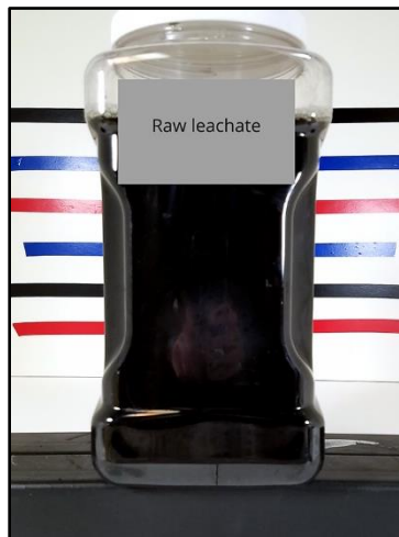
Leachate before treatment.
