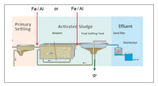
Electrocoagulation replaces the FE/AL chemicals shown above by dissolving pure metal ions directly into the water.<sup>2,3</sup>
