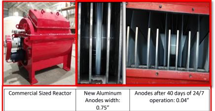
Rotational anodes were fully consumed after 40 days of 24x7 operation without passivation and without sludge buildup within the reactor.
