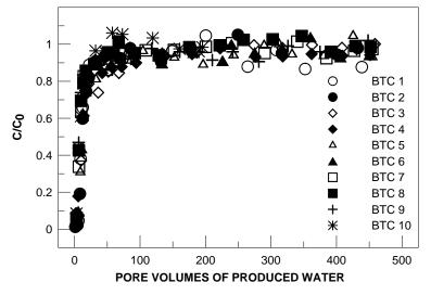
Figure 1. Repetitive sorption of benzene on and SMZ column, with air sparging between breakthrough curves (BTCs) (Ranck, in press). Similar results were seen for toluene, ethylbenzene, and xylenes.
