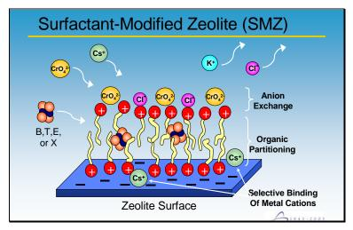
Although this appears complicated, the important part is the zone of organic partitioning. The surfactant molecules (red balls with yellow tails) are ion-exchanged to the clinoptilolite surface. In this illustration, the hydrophobic tails have formed a bilayer on the surface as the result of hydrophobic attraction between tail groups. BTEX compounds (left) are sorbed by the hydrophobic zone. Air stripping can remove these volatile organics from the hydrophobic zone easily.
