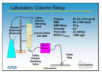
The set-up in the laboratory.
