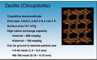
The base material for the sorbent in the SMZ/VPB system is clinoptilolite zeolite. This mineral is mined in areas such as southwest New Mexico, central Idaho, and Wyoming. It is abundant, inexpensive, and frequently used as an ion-exchange medium or molecular sieve-filter medium in water treatment processes.
