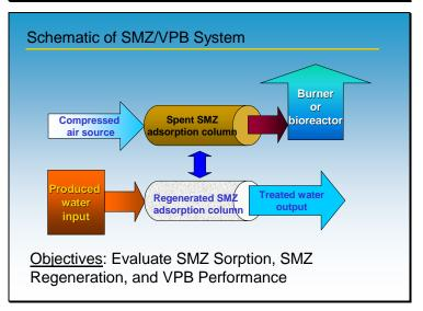
Input water flows through one or more SMZ adsorption columns. Treated water is output. In a multicolumn setup, one column at a time would be removed from the flow for regeneration by air sparging. The sparged air (from an inexpensive compressor) would be sent to a Vapor Phase bioreactor to remove BTEX compounds. The regenerated column would be returned to use and another column cycled out for regeneration.
