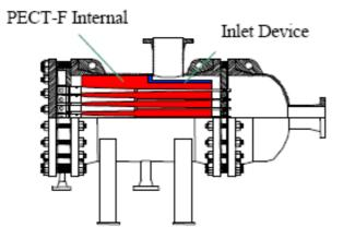
Figure 7. Conventional deoiling hydrocyclone vessel equipped with PECT technology
