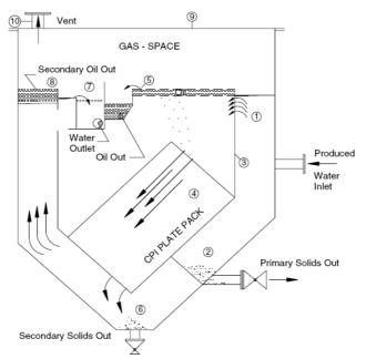
Figure 4. Cross section showing flow pattern of a skim pile [4]
