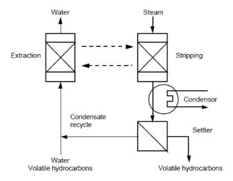
Figure 12. MPPE extraction/ stripping system [27]
