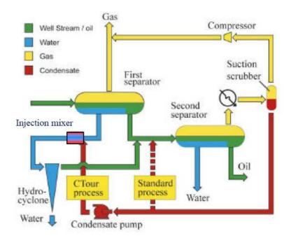
Figure 11. Flow diagram of the CTour process [11]
