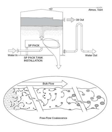
Figure 6. Principles of operation of an SP Pack [4]
