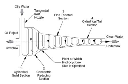
**Figure 9.** Principles of operation of a hydrocyclone: 1) cylindrical swirl chamber 2)concentric reducing section 3) fine tapered section 4) a cylindrical tail section [4]
