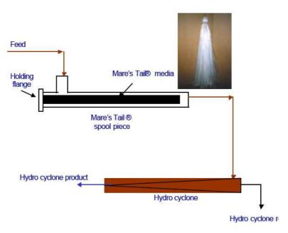
Figure 8. Principle of operation of Mare's Tail [11]
