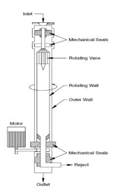
Figure 10. Centrifuge system for oil-water separation [4]
